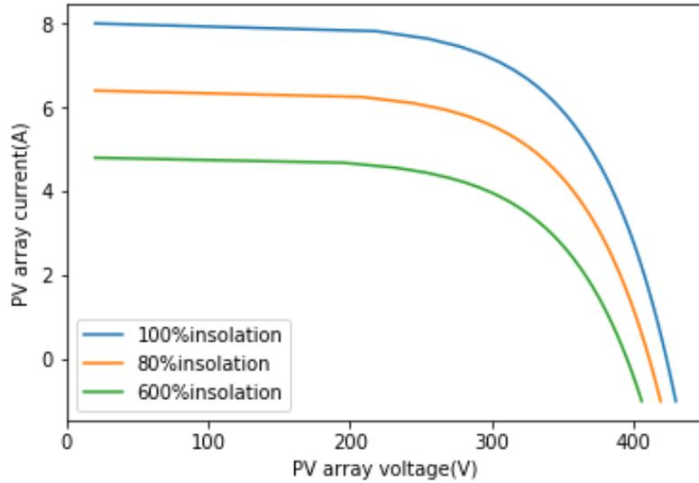
Fig. 2. VI characteristics of PV panel for different insolation levels
