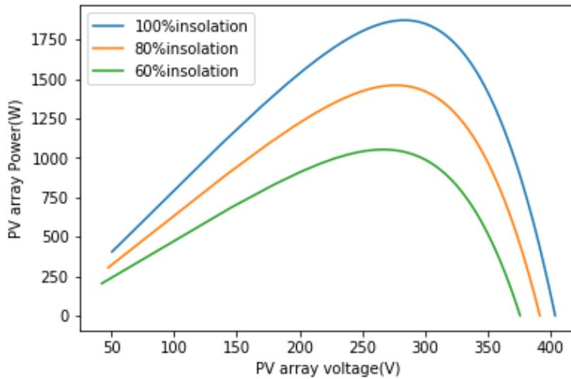
Fig. 3. PV characteristic of solar panel for different insolation levels
