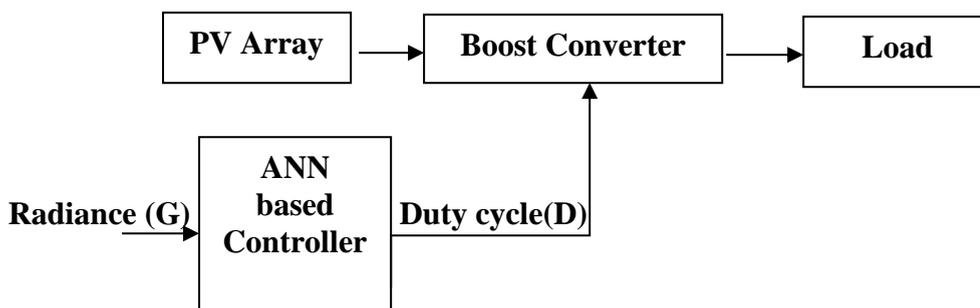
Fig 1: ANN based MPPT controller utilizing G & D as inputs.
